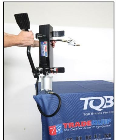
3. While holding the pump vertically depress the release valve pedal and allow the ram to retract to fully retracted position.
